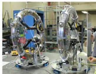
Backplane metallic object. RING testbed for WPT/FF oriented to ISS
