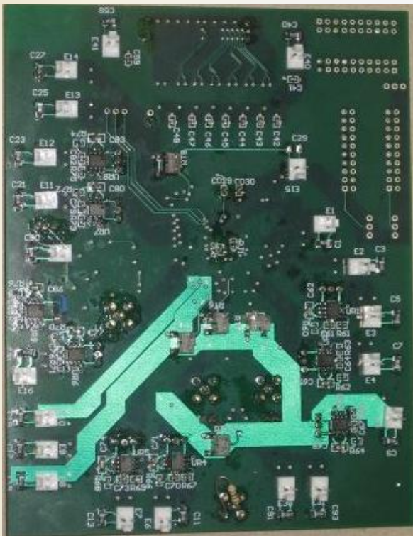
DC Regulators on bottomside of the PCB
