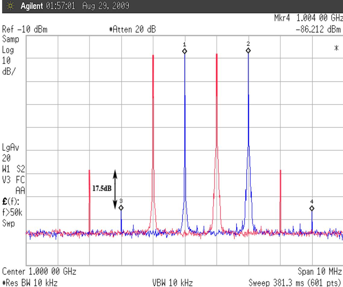
Two-tone test measurements with -16.5 dBm input power per tone at 1GHz with  $\Delta f = 2$  MHz
