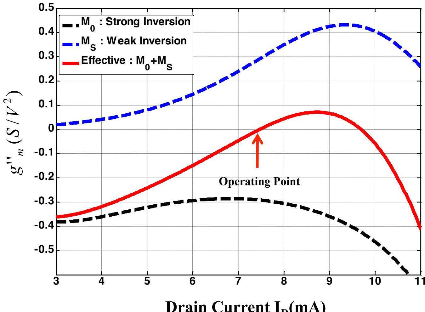
➤ Poor Large signal linearity ( $P_{1dB}$ )
