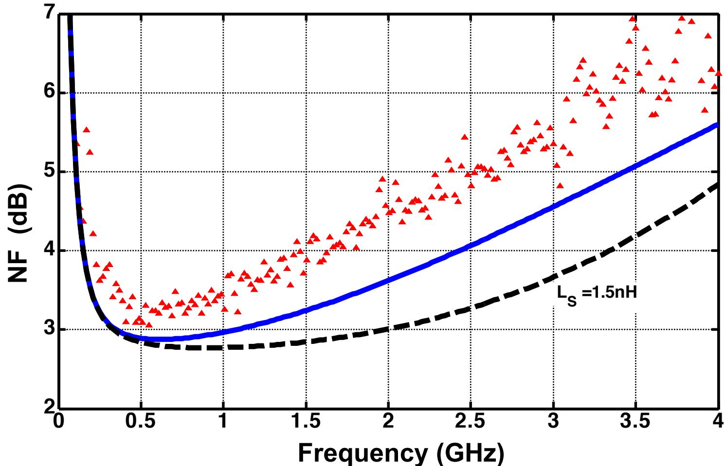
NF of LNTA (lines: simulations; markers: measurements,
