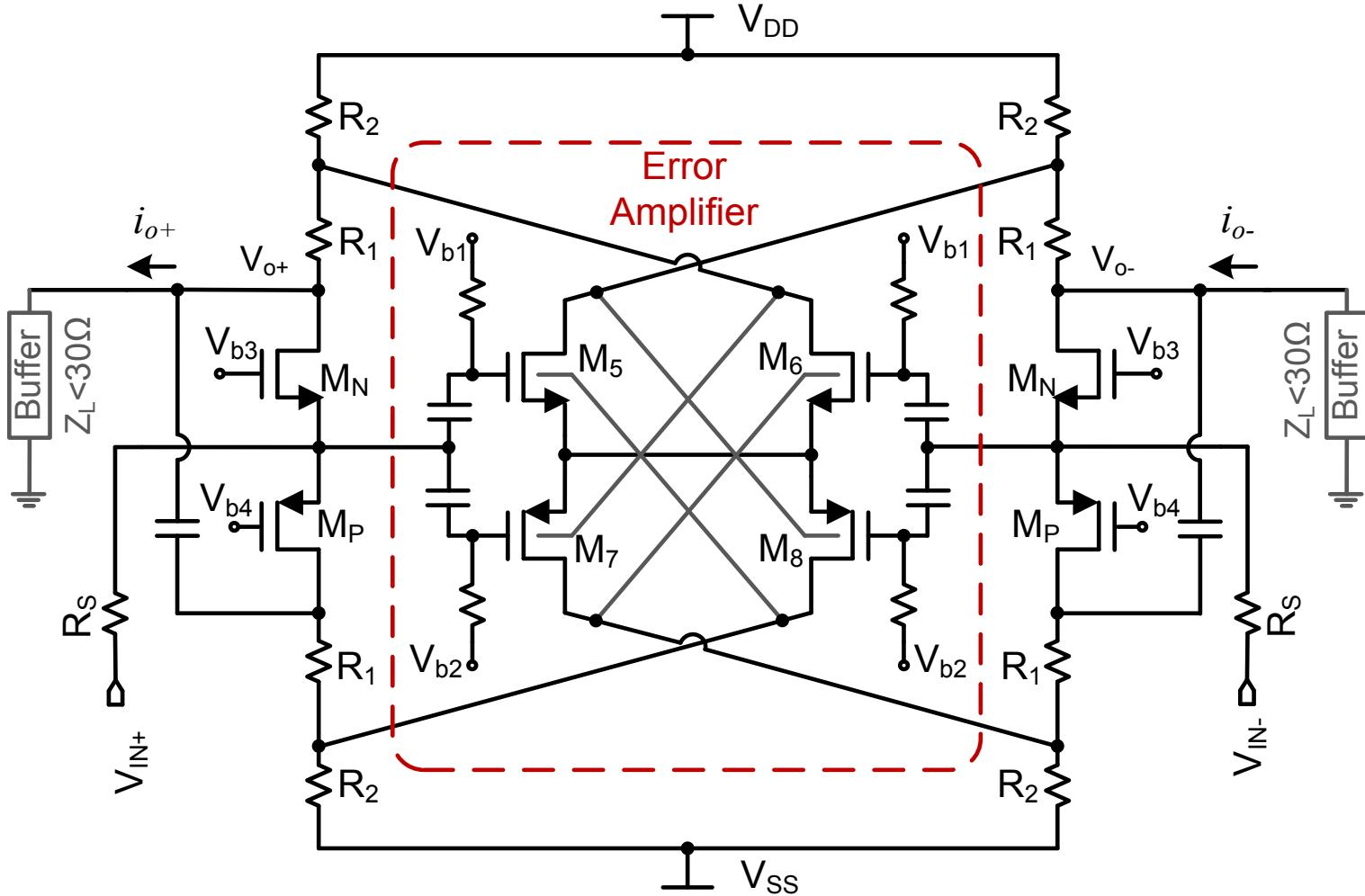
**Bulk driven EA:** transistor sizes and currents are scaled down to maintain the value of the original transconductance
